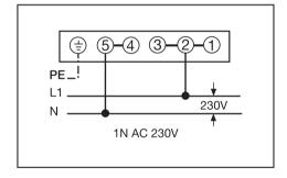
When replacing the cable supplied with another cable or changing the connection, only cable type H 05 VV-F with a suitable cross-sectional area (CSA) may be used (available from Miele Spare Parts).
